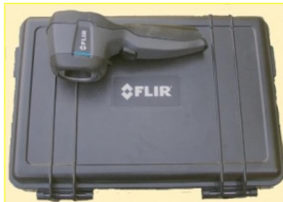
Figure 3. The FLIR i7 camera used in this project.
