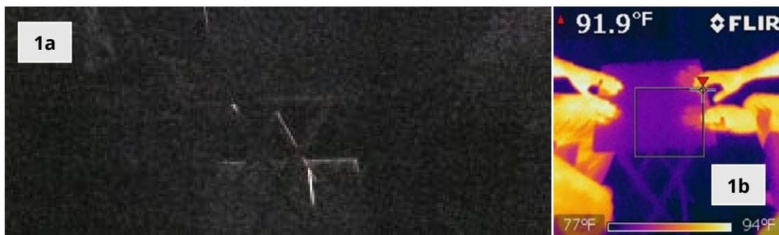
Figure 1. Comparison of images from a standard visible light camera using a long exposure (1a) and a thermal image (1b). Both images were collected under the same low-light conditions. Heat transfer can be seen on the table top in the thermal image.
